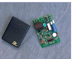
There is a built-in time delay circuit in the Quik-Chek receiver to keep the emergency light lamp heads on for a preset period of time. This time delay has an adjustable setting of 1 to 90 seconds or minutes.
